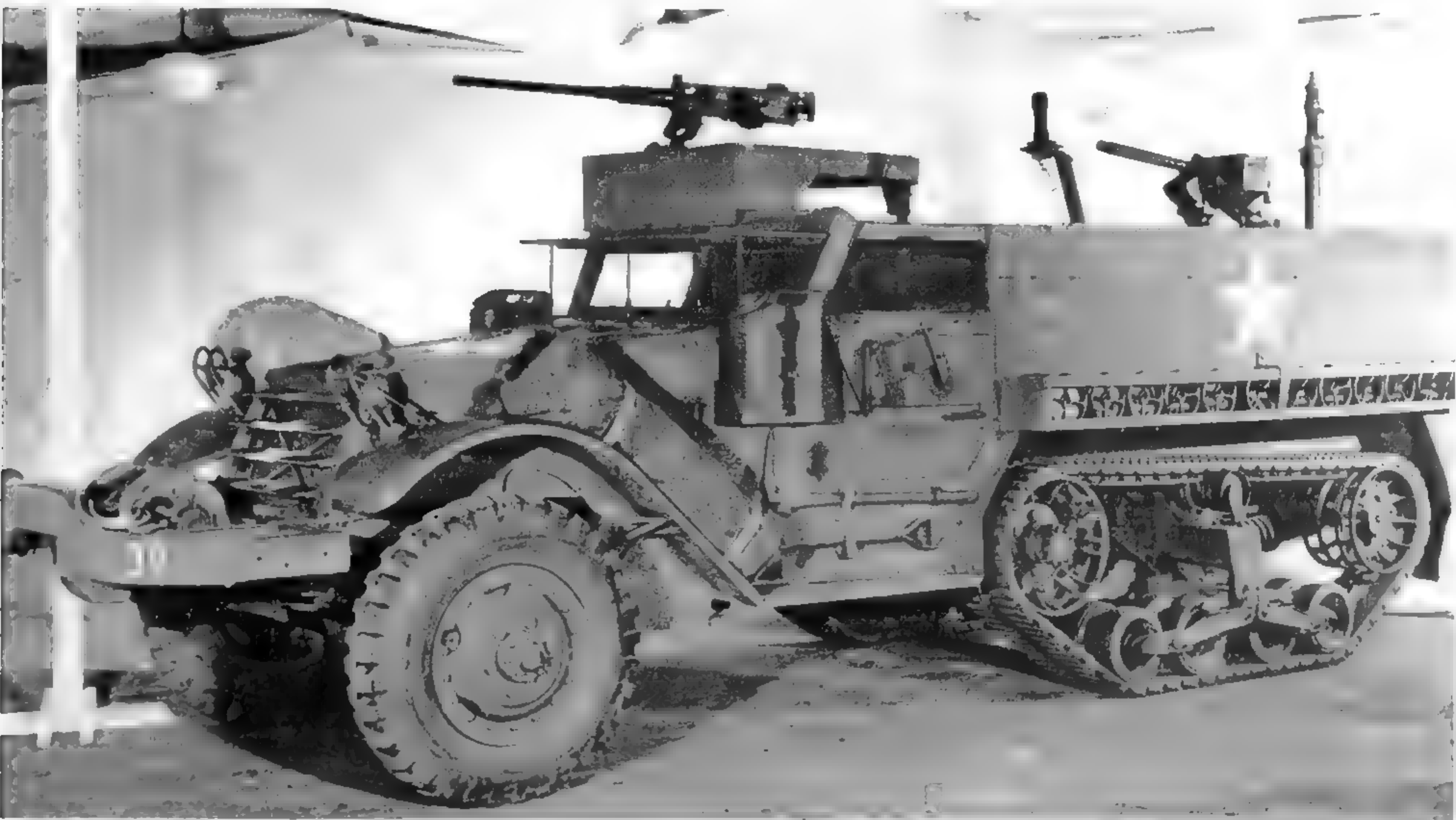
This February 1944 photo of an M9A1 halftrack with winch was taken at the Engineering Standards Research Laboratory. Externally, the M5A1 and M9A1 were very similar, but the interior arrangements were different. (U.S. Army photo)
